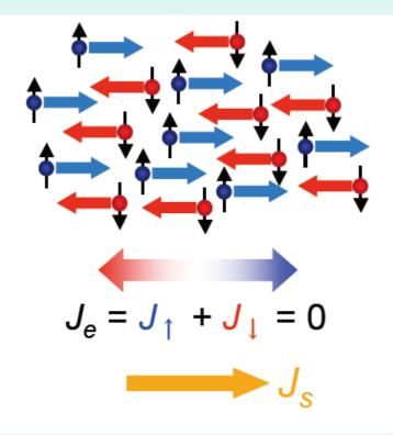
If ↑spin current moves toward right, and if ↓spin current moves toward left, no net charge current flows, while a net spin current J<sub>↑</sub>-J<sub>↓</sub> flows from the left to right.
