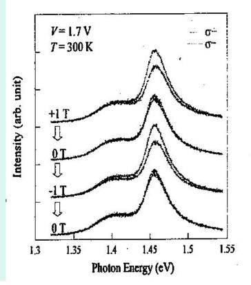
Magnetic field dependence of EL spectra for different chirality of circularly polaized light
