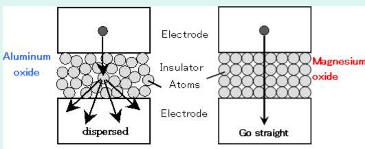
(a) Conventional device Using aluminum oxide (amorphous). Electrons are scattered due to disorder atom arrangement. (b) Novel single-crystal device Using magnesium oxide (single-crystal). Electrons can move straight without suffering dispersion.
