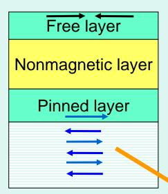
Important point of this invention is a use of the exchange bias effect introduced by coupling with antiferromagnetic substrate.
